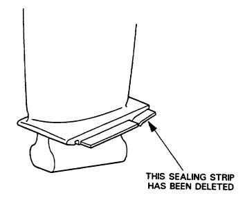
HP compressor blade sealing strip - Stages 4 and 5 (Typical) Fig.1
