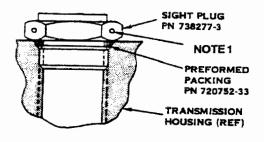
SECTION A-A ENLARGED (SIGHT PLUG INSTALLED)
