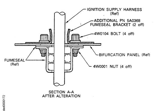
Fumeseal Installation on the Bifurcation Panel Fig.1 Sheet 2 of 2
