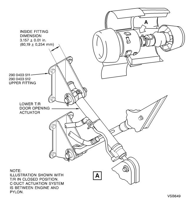
Lower Thrust Reverser Half Opening Actuator Pylon Upper Fitting Inspection Figure 1
