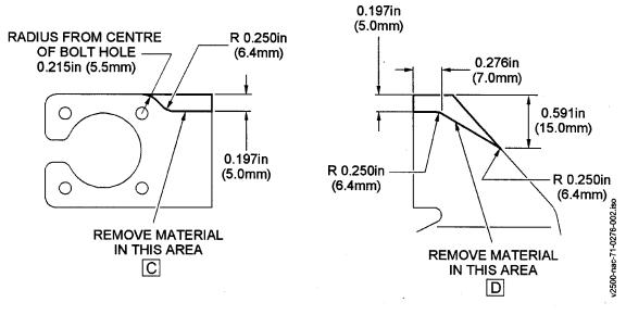
Rework of the Bracket and Fire Detection Harness (System B) Figure 1, sheet 2 of 3
