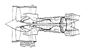
REMOVE THE PN 2A0160 STAGE 2 HPT BLADE RETAINING PLATE (1 Off) AND INSTALL THE PN 2A1813 STAGE 2 HPT BLADE RETAINING
