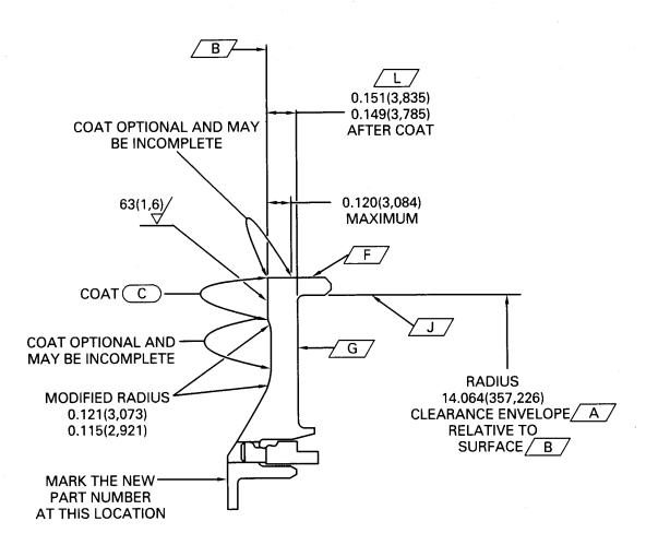
SECTION A-A ROTATED SHOWING AFTER COAT REQUIREMENTS
