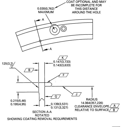
NOTE:UNLESS DIFFERENTLY SPECIFIED ALL DIMENSIONS APPLY WHEN SURFACE GIS  $O02 \atop (0,051)$  AND CLEARANCE ENVELOPE A IS HELD, IN A FREE STATE OR WITH A FIXTURE. THE FIXTURE CAN ONLY TOUCH THE PART ON SURFACES GUNLESS DIFFERENTLY SPECIFIED ALL SURFACES GUNLESS DIFFERENTLY SPECIFIED BREAK EDGES 0.003 - 0.015(0,08 - 0,38)
