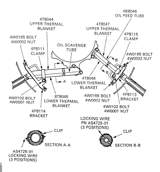
Assembly of Insulation Shielding Fig.2
