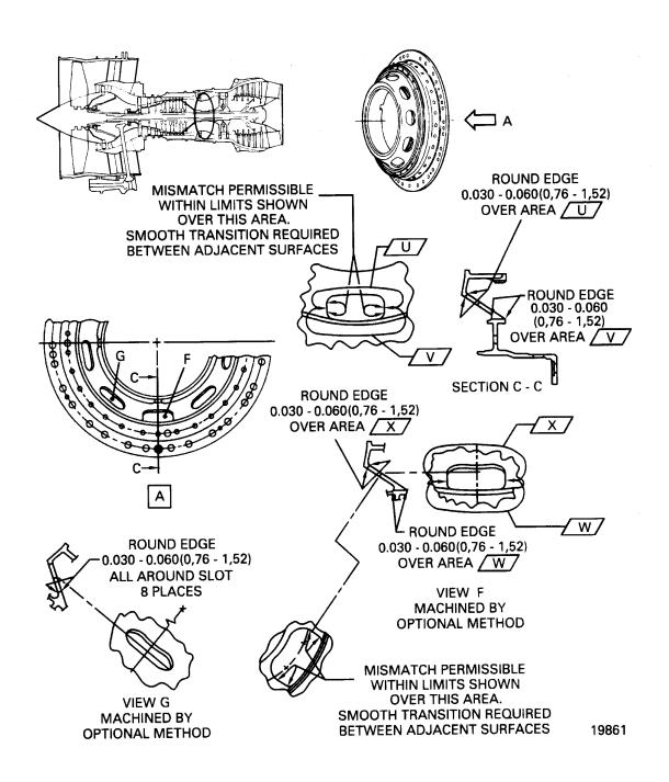
Modification of No.4 bearing support assembly Fig.4
