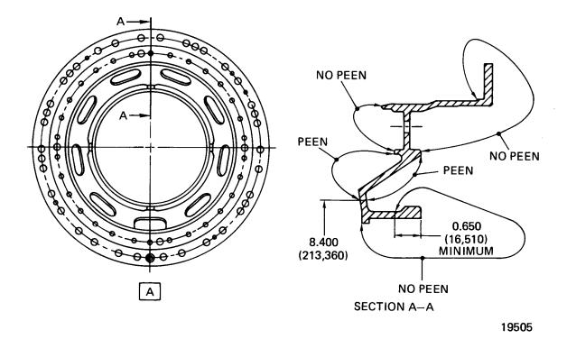
$\begin{array}{c} \textbf{Modification of No.4 bearing support assembly} \\ \textbf{Fig.5} \end{array}$
