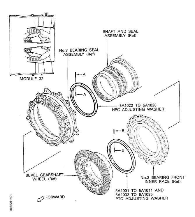
Location of the HPC and the PTO adjusting washers Fig.1
