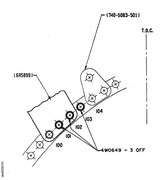
View on arrow A (see Figure 3) showing location of cooling air deflector - After alteration
