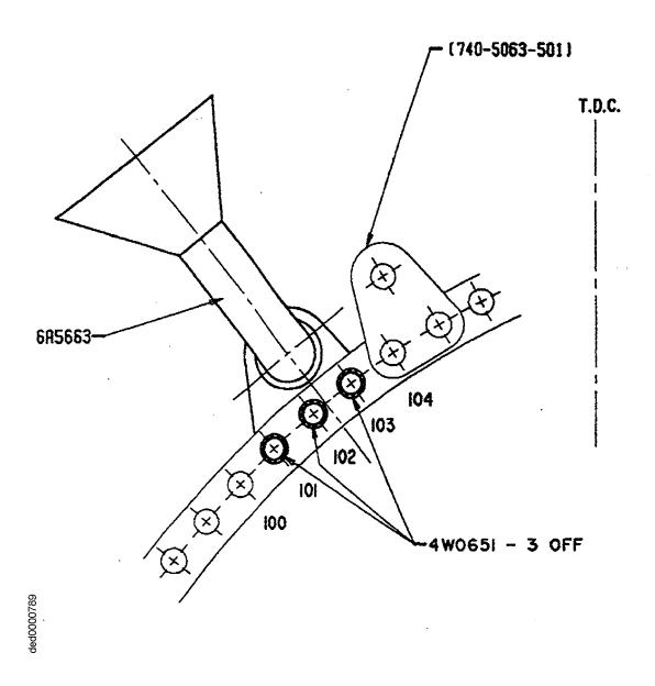
View on flange FK looking forward, showing location of cooling air deflector - Before alteration
