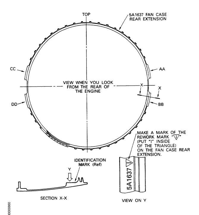
Rework of the Fan Case Rear Extension Fig.1
