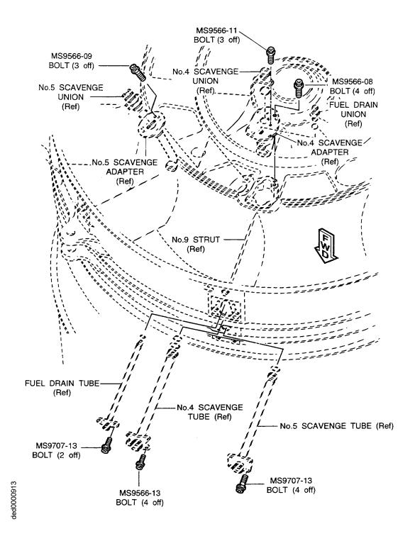
Install the LPC Intermediate Case Module Attaching Bolts Fig.1
