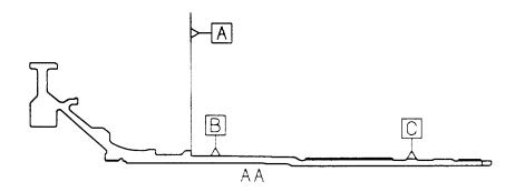
BASIC SECTION THROUGH HP COMPRESSOR REAR SHAFT
