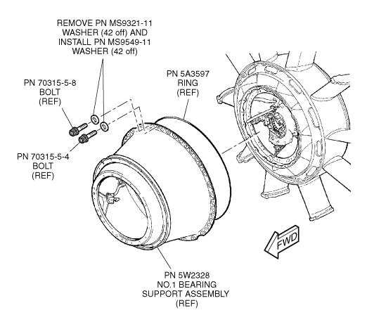
Location of the Washer that connects the No.1 Bearing Support to the Fan Frame Figure 1
