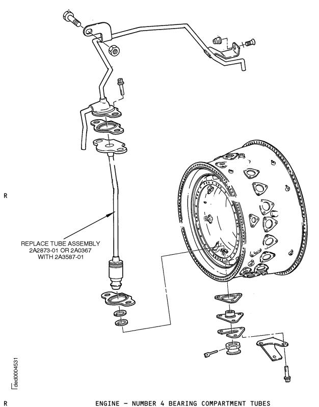
ENGINE - NUMBER 4 BEARING COMPARTMENT TUBES Figure 1
