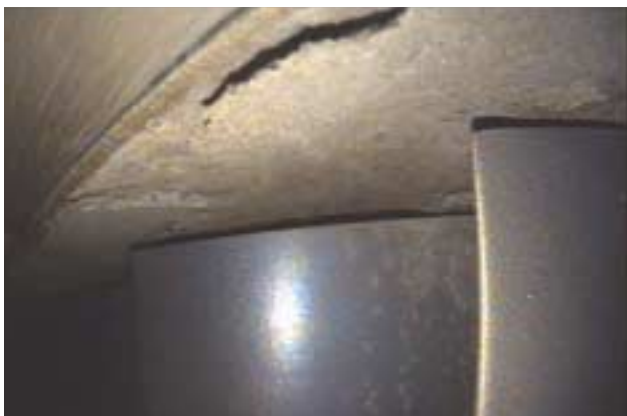
Fig 5 – Examples of corrosion related, lifting, blistering, bulging or swelling of topcoat surface
