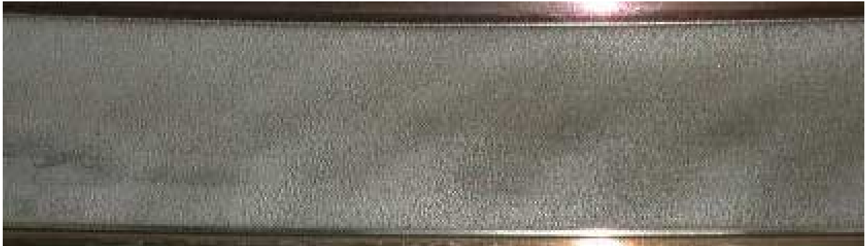
Fig 1 – Uniformly sound topcoat surface
