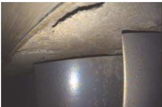
Figs 5 & 5a – Examples of corrosion related pitting, lifting, flaking or blistering of topcoat surface
