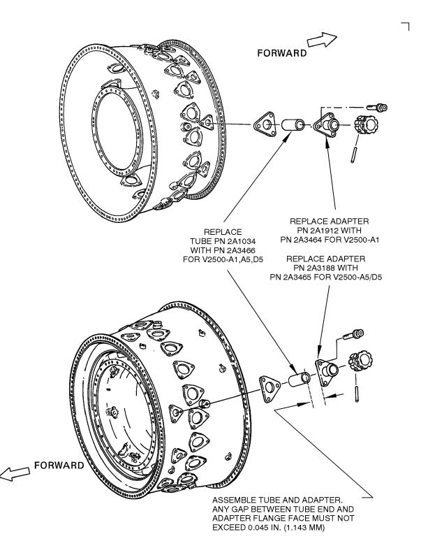
NUMBER 4 BEARING COMPARTMENT TUBE AND ADAPTER LOCATION REF. CATALOG SEQUENCE NO. 72-40-20-FIG. 06
