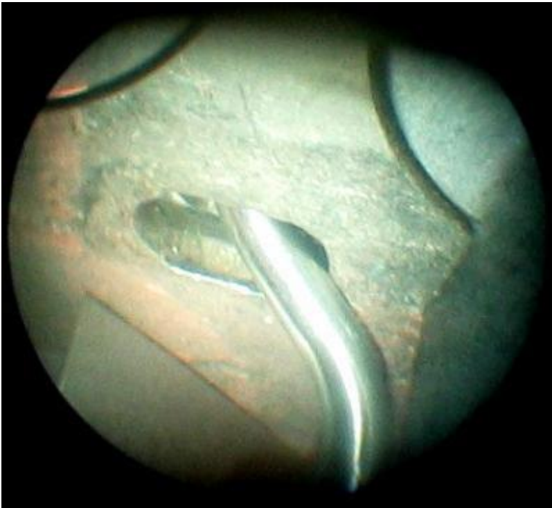
View looking outwards at tooling port in casing. Verification of correct probe parking. Note position of guide tube at edge of port
