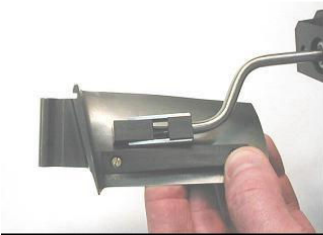
Ultrasonic calibration. Note position of probe approximately 5.0mm from notch Fig. 8
