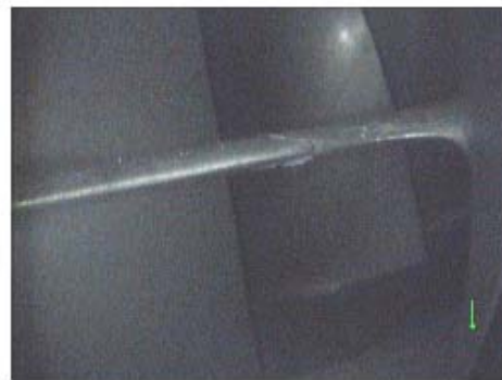
Advanced Aligned Irregular Wear to same pair of blades
