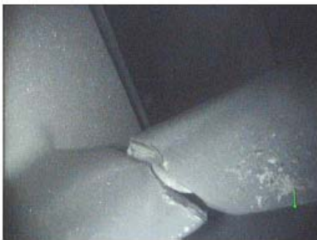
Advanced Aligned Irregular Wear to same pair of blades
