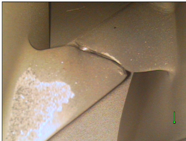
Aligned Irregular Wear
