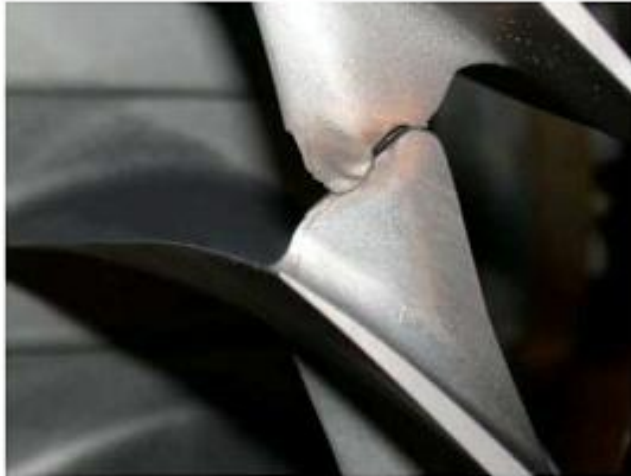
Severe Irregular Wear Material Missing and Cracking
