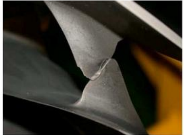
Severe Irregular Wear Material Missing and Cracking
