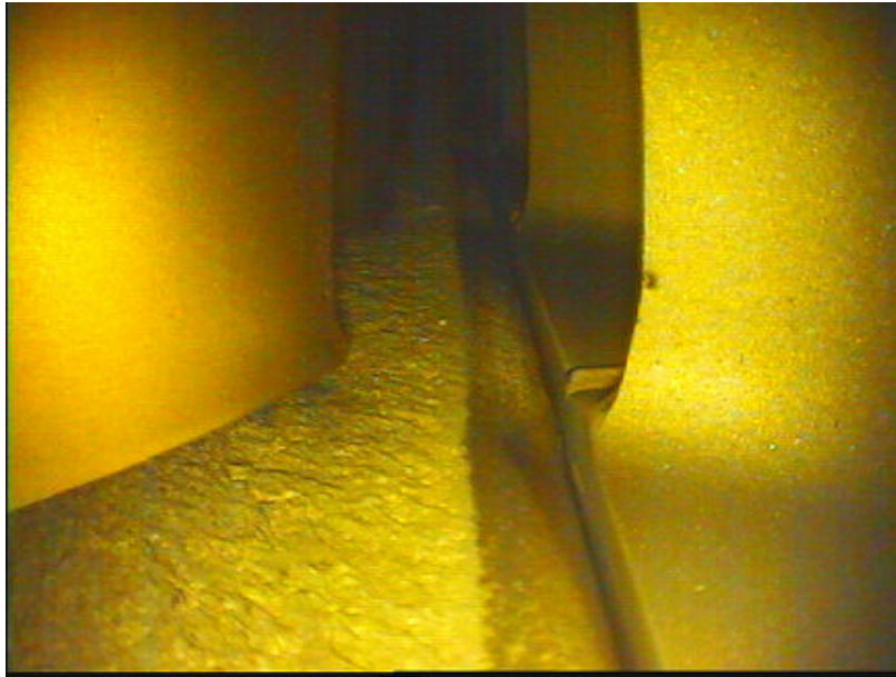
R HPC stage 6 stator vane with nick at the T/E, dimension of the nick R 0.014 in. (0,36 mm), no material removal allowed R Figure 6
