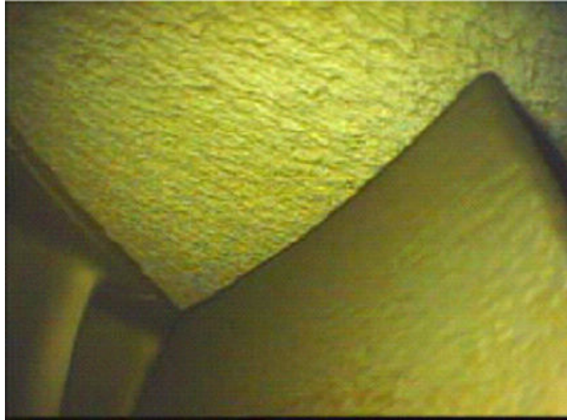
HPC stage 6 rotor blade without blade tip erosion Figure 10
