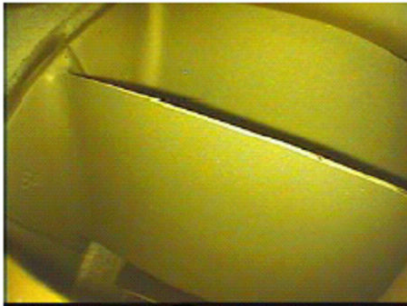
HPC stage 7 stator vane with a thin T/E which remains straight Figure 9
