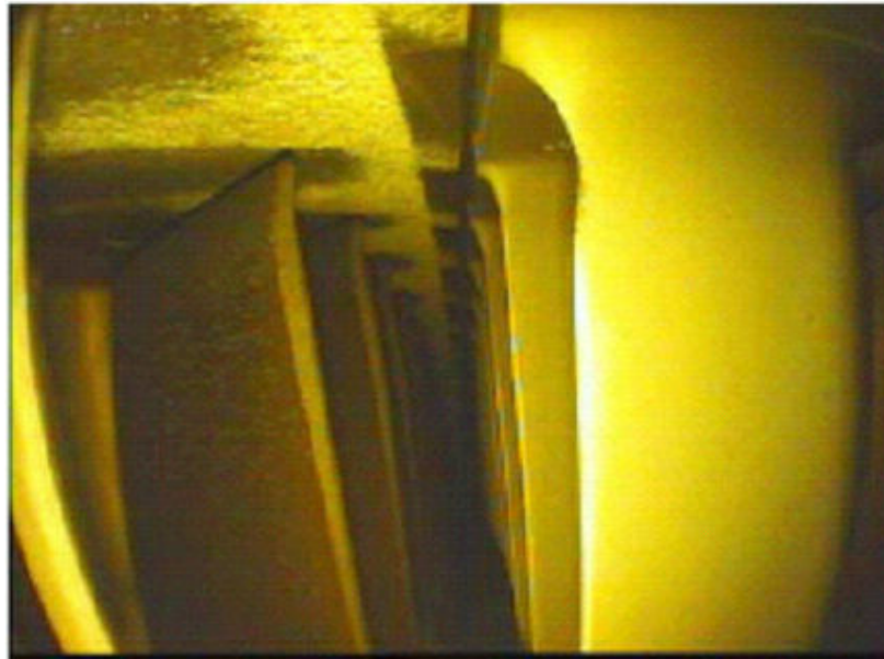
R HPC stage 6 stator vane; smooth loss of material without a jagged T/E R Figure 7
