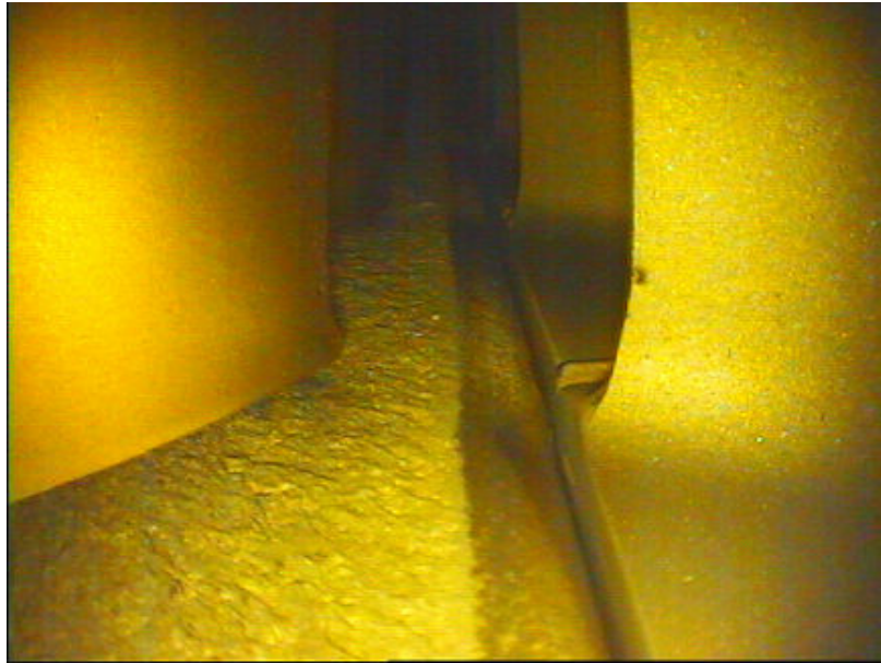
R HPC stage 6 vane with nick at the T/E, dimension of the nick R 0.014 in. (0,36 mm), no material removal allowed R Figure 7
