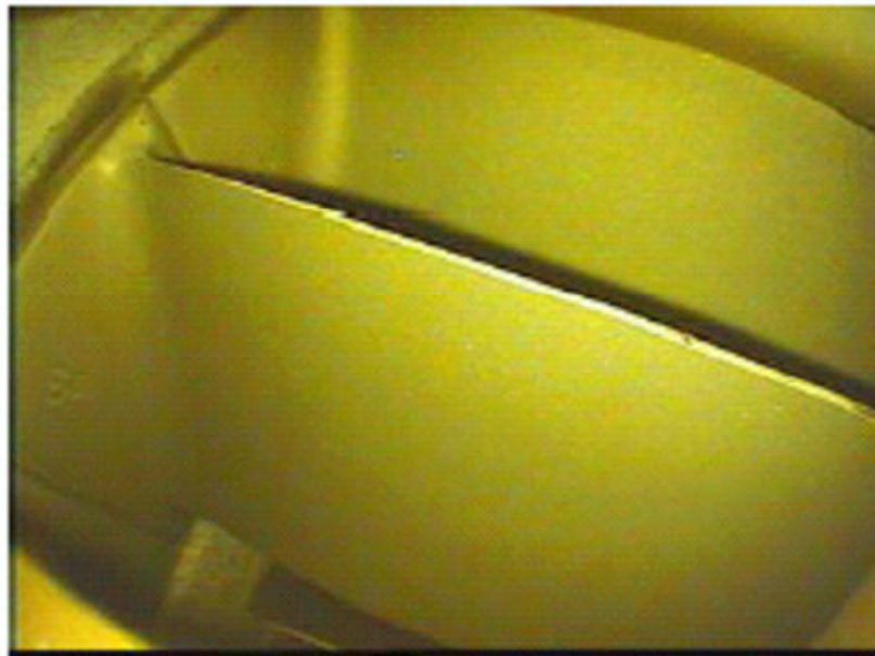
HPC stage 6 vane with a thin T/E which remains straight Figure 10
