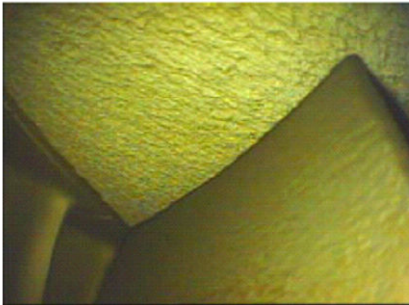
HPC stage 6 blade without blade tip erosion Figure 11
