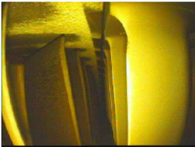
R HPC stage 6 vane; smooth loss of material without a jagged T/E R Figure 8
