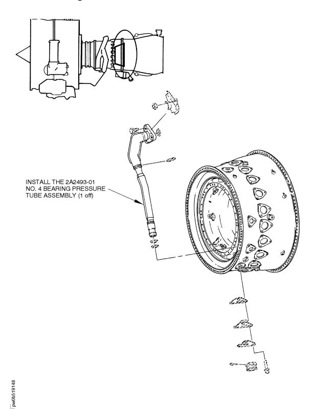
LOCATION OF THE NO. 4 BEARING PRESSURE TUBE ASSEMBLY Figure 1
