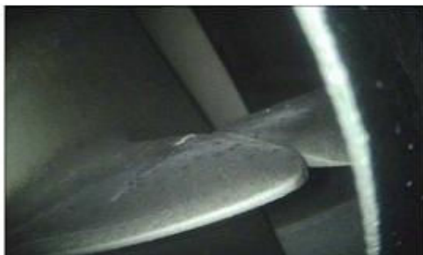
CLAPPERS WITH GOOD ALIGNMENT NO OBVIOUS WEAR
