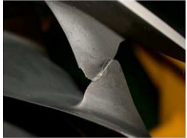
Severe Irregular Wear Material Missing and Cracking
