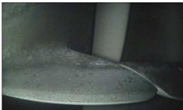
CLAPPERS WITH GOOD ALIGNMENT NO OBVIOUS WEAR
