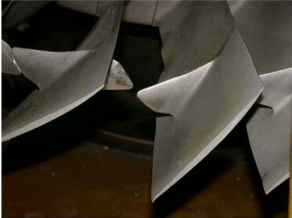
Clappers Totally Mis-Aligned and Blade Bent Result of Bird Strike
