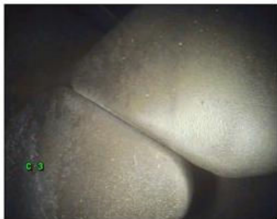
CLAPPERS WITH GOOD ALIGNMENT NO OBVIOUS WEAR
