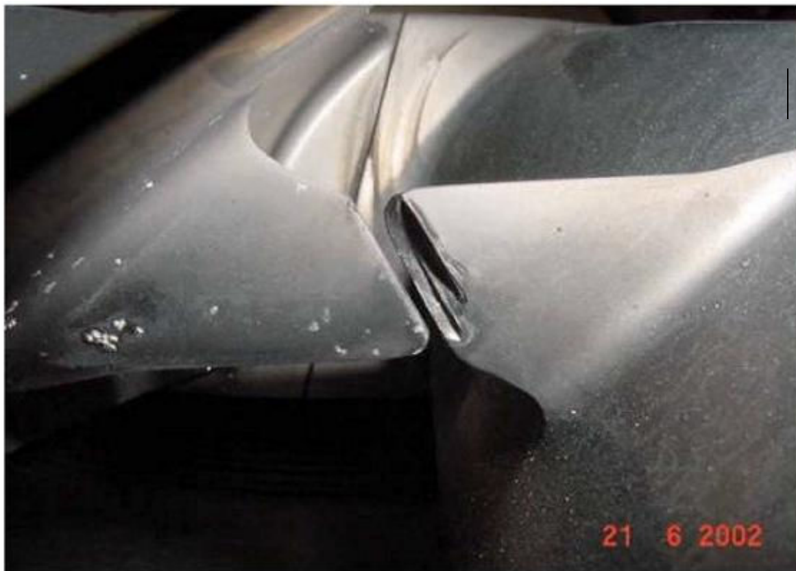
Aligned Stepped Wear
