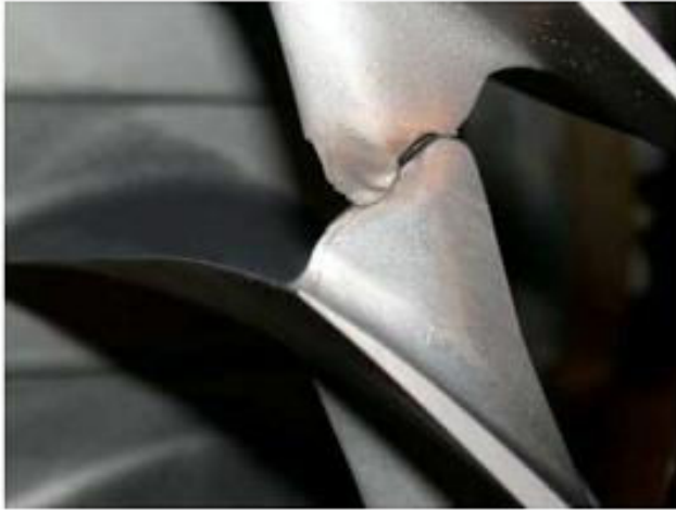
Severe Irregular Wear Material Missing and Cracking
