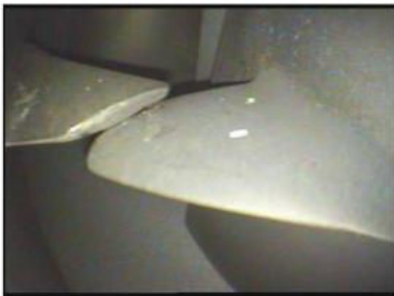
Shingled as a Result of Bird Strike
