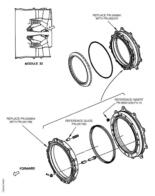
NO. 3 BEARING REAR OIL SEAL ASSEMBLY FIGURE 1
