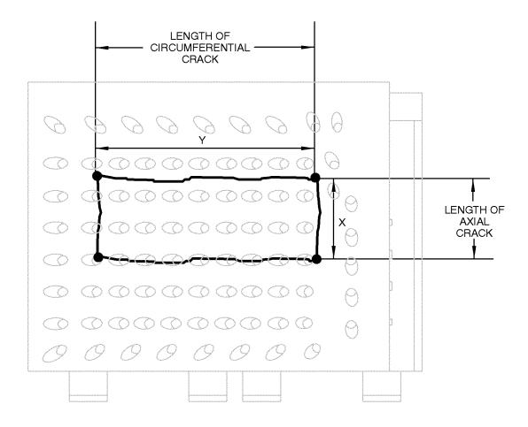
NOTE: IN THIS EXAMPLE, MAXIMUM LENGTH IS Y, BECAUSE THE CIRCUMFERENTIAL CRACK IS LONGER THAN THE AXIAL CRACK.
