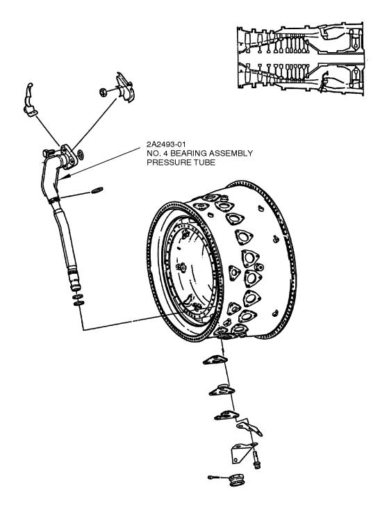
LOCATION OF THE NO.4 BEARING ASSEMBLY PRESSURE TUBE 72-42-20 FIGURE 1
