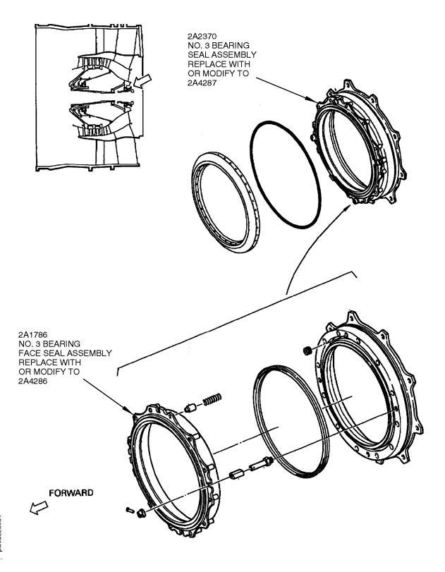
Location of the No. 3 Bearing Seal Assembly 72-32-25 Figure 1
