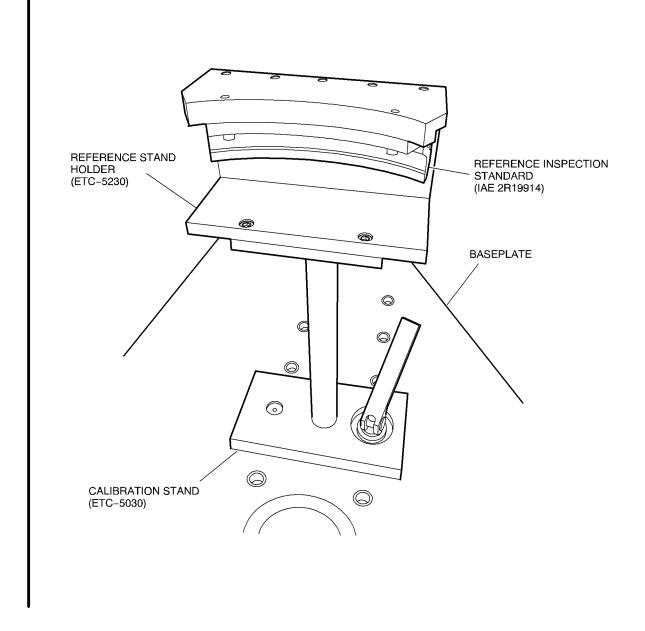
$\underline{\text{NOTE:}}$  FOR CALIBRATION, THE SECOND SET OF HOLES IN THE ETC-2000 BASEPLATE IS USED.
