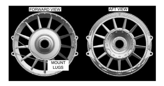
PART GRAPHIC SHOWING MOUNT LUG LOCATIONS FROM FORWARD (LEFT) AND AFT (RIGHT)
