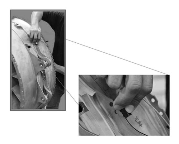
PROBE POSITIONED SUCH THAT THE SENSOR TRANSVERSES SIDE FACE FIGURE 6
