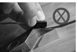
PROPER PROBE TRAVEL WITH SENSOR IN LEADING POSITION AND CABLE IN TRAILING POSITION IS SHOWN IN LEFT GRAPHIC. IF THE PROBE TRAVELS SUCH THAT THE SENSOR APPROACHES THE EDGE TRANSITION AS SHOWN IN THE RIGHT GRAPHIC, GEOMETRY NOISE IS MORE SEVERE AND WILL LEAD TO UNINSPECTABLE AREAS.
