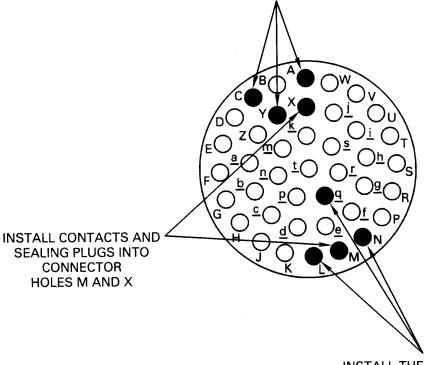
INSTALL THE JUMPER PIN FROM CONNECTOR HOLE M INTO CONNECTOR HOLE <u>q</u> (This is one of a three pin jumper)
