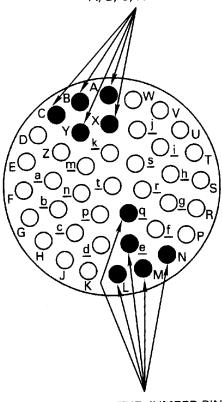
INSTALL THE JUMPER PINS IN CONNECTOR HOLES e, L, M, N AND 9
