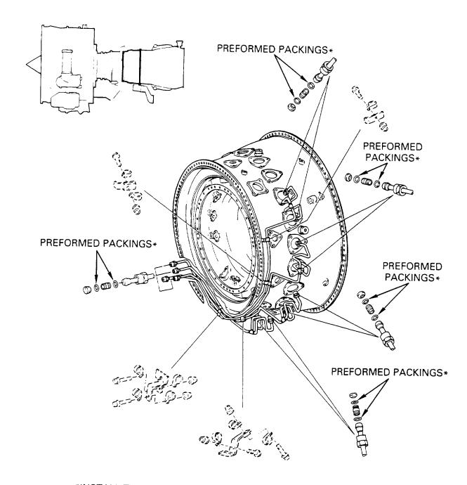
\*INSTALL THE AS3209 - 010 PREFORMED PACKINGS (24 Off)
