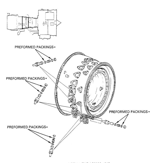
\*INSTALL THE AS3209 - 010 PREFORMED PACKINGS (18 Off)
