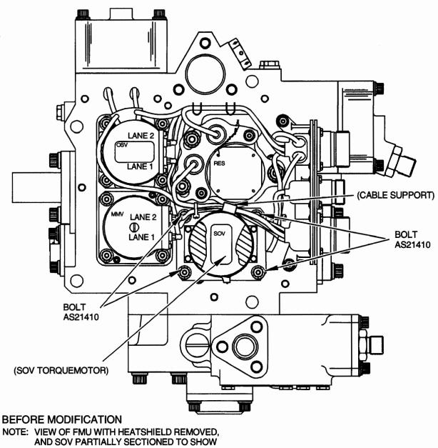
AND SOV PARTIALLY SECTIONED TO SHOW CURRENT BOLTS SECURING SOV TORQUEMOTOR TO FMU BODY.
