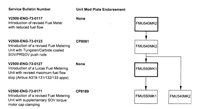
\* This family tree is not intended to represent the combination of modifications fitted to units in service
