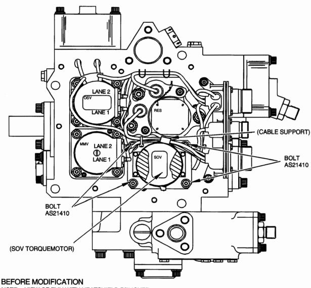
NOTE: VIEW OF FMU WITH HEATSHIELD REMOVED,
