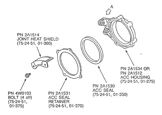
Assembly of new HPT manifold joint and support parts Fig.4 (Sheet 1 of 2)
