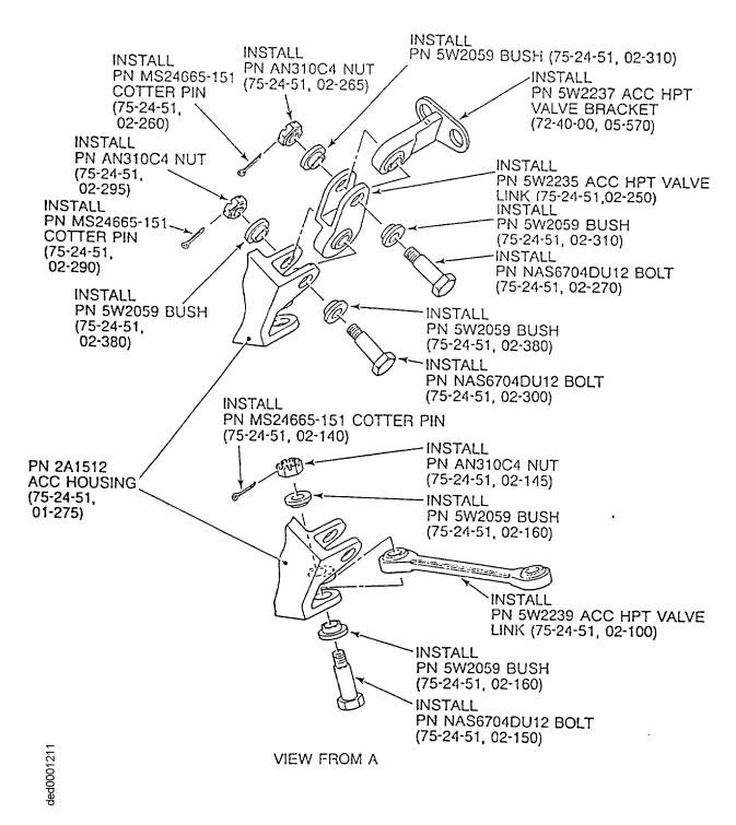
Assembly of new HPT manifold joint and support parts Fig.4 (Sheet 2 of 2)
