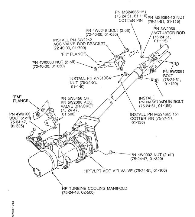
Installation of HPT/LPT ACC Air Valve Fig.6 (Sheet 1 of 2)
