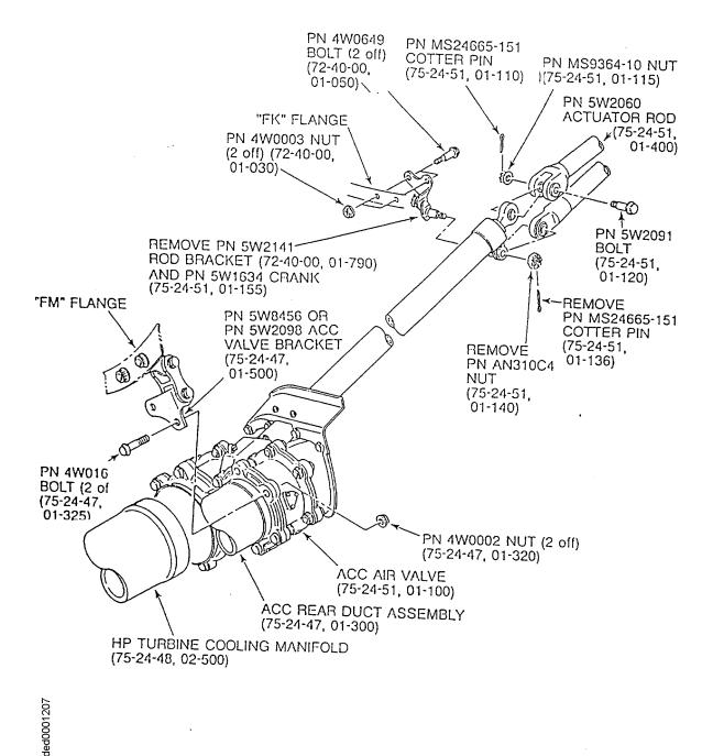
Removal of HPT/LPT ACC Air Valve Fig.1
