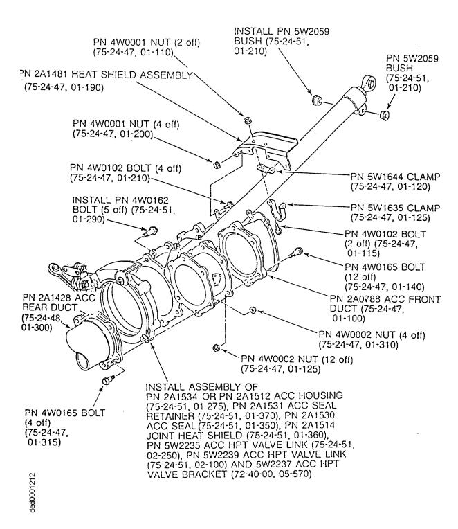
Installation of ACC system parts to HPT/LPT ACC Air Valve Fig.5
