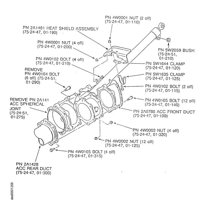
Removal of ACC system parts from HPT/LPT ACC Air Valve Fig.2
