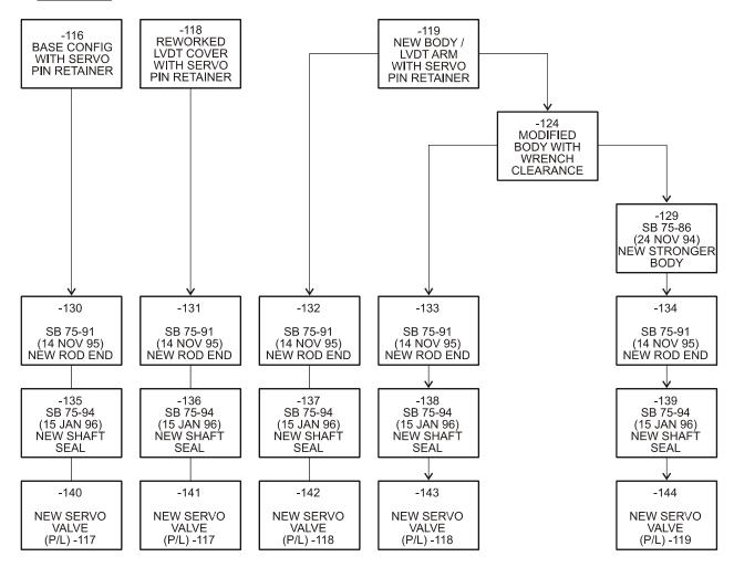
NOTE: THIS FAMILY TREE INCLUDES ONLY THE ACTIVE CONFIGURATIONS OF BASIC PART NUMBER 5860017 THAT CAN BE UPGRADED WITH THE NEW SERVO. CONFIGURATIONS NOT LISTED MUST INCORPORATE THE APPROPRIATE IMPROVEMENTS THAT CONFORM TO THE CONFIGURATIONS SHOWN.
