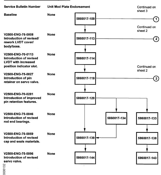
V2500-A1 ACC Actuator Family Tree Fig.1 (Sheet 1 of 3)
