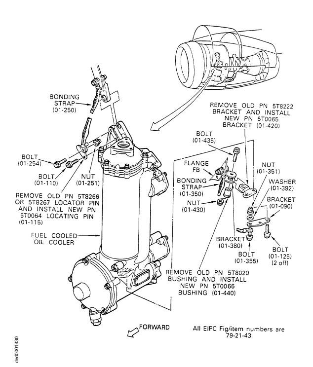
FCOC Mount Bracket, Pin and Bushing Fig.1
