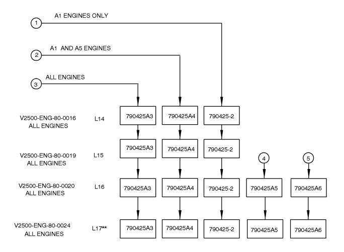
\*\*THE L NUMBER ONLY ADVANCES TO L17 WHEN SPP SB 80-2520 IS ACCOMPLISHED PAET NUMBER IS CHANGED WHEN SPP SB 80-2521 IS ACCOMPLISHED
