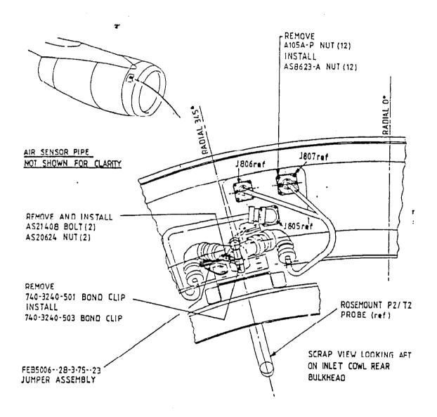
Removal and Replacement of the Bonding Clamp and Connector Nuts Figure 1  $\,$
