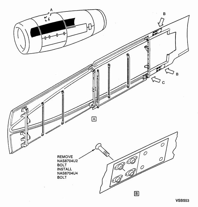
Replace the Pylon Apron Bolts - Left Nacelle Figure 1 (sheet 1)
