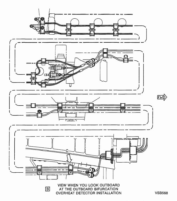
Overheat Detector Harness Installation Modification Figure 1 (Sheet 2)
